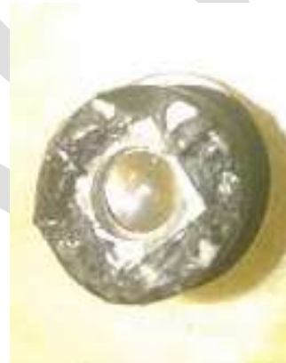
Figure.4 Infrared filter from the web camera.
