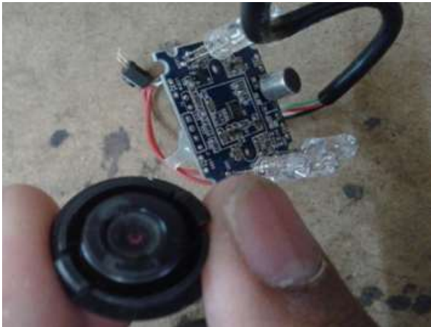
Figure.3 Lens assembly inside camera
