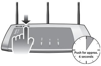
As soon as the "WLAN" LED begins flashing, enable the WPS function on the other WLAN device, either by pressing a button or in the device's user interface (depending on the device). Activation must be started within two minutes.
