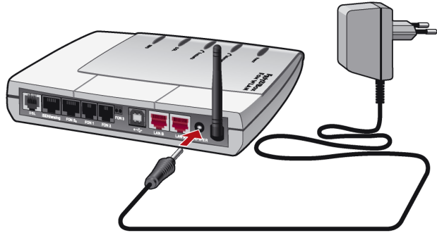
Connecting FRITZ!Box Fon WLAN to the power supply
