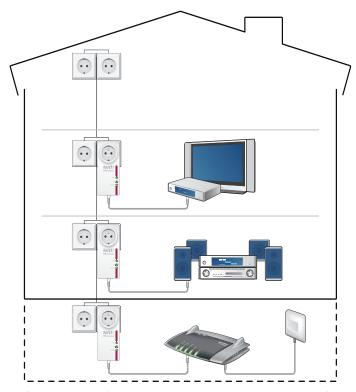
With FRITZ!Powerline 520E you can integrate your TV and your stereo system into your network. When the network is connected with the Internet, the TV can use services like video on demand, IP TV or services available in the Internet like You-Tube and Flickr. The stereo system can receive web radio stations. Both devices also enjoy access to the collections of photographs, videos and music available in the home network, which can be accessed on network storage.
