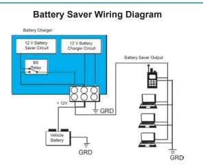
**Battery Saver Operation:** When the battery charger is operating, the vehicle's accessories are powered by the 12V battery saver circuit, internal to the charger. When the charger is powered off, a relay inside the charger switches the vehicle accessories directly to the battery.
