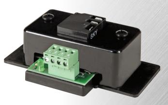
to the same terminal de-energizes the relay and turns the load "OFF". Both inputs may come from the same switch or from any number of switches in parallel. A load may be turned "ON" from one location and turned "OFF" from another. An output signal on the Alternate Action Relay operates a remote indicator to indicate when the load is energized.
