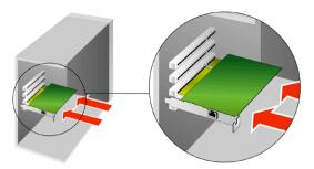
Inserting the FRITZ!Card PCI into the PCI slot
