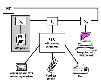
Typical configuration of a point-to-multipoint ISDN line
