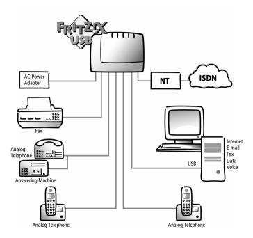
Computer and analog terminal equipment connected to an ISDN line using FRITZ!X USB
