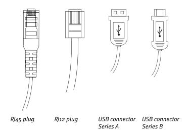
The ISDN cable supplied with FRITZ!X USB has an RJ45 plug at each end. The power cord also has a RJ45 plug at one end.
