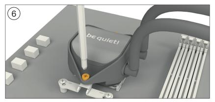
Place the CPU block centrally over the short AMD mounting brackets (5), such that these allow the CPU block to be screwed down. For this you can use a normal crosshead screwdriver. Next connect the pump and the LED illumination to the SATA adapter (18).
