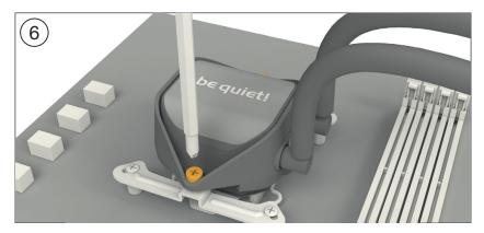
Place the CPU block centrally over the Intel mounting brackets (4), such that these allow the CPU block to be screwed down. For this you can use a normal crosshead screwdriver. Next connect the pump and the LED illumination to the SATA adapter (18).
