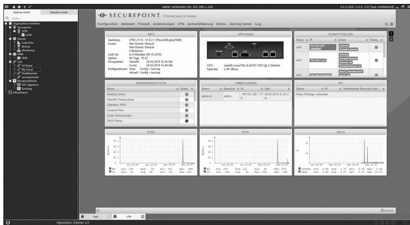
There is the possibility of direct SSH connections to individual firewalls. The usual settings of the administration web interface can be accessed here. The Client of the Operation Center is installed locally on a computer.
