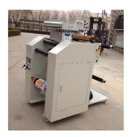
Maximum unwinding diameter:700 mm Double side walls for load bearing Pneumatic paper loading Sensor for label count from Taiwan Sensor for label length from Taiwan Separate ST web guide from Italy, with pneumatic clamps 9 sets of scissor knives
