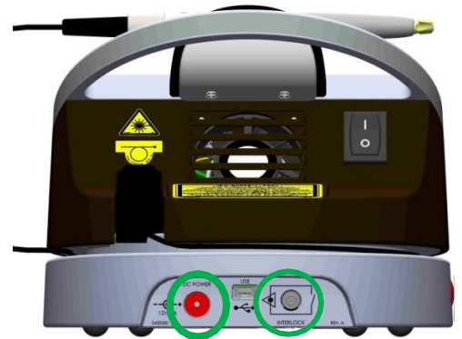
Figure 6.1: Power Switch, DC Power Input, Remote Interlock
