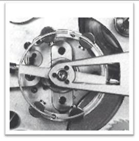
The integral balance called the Guillaume balance, which eliminates errors due to thermal variations, is used for high-grade watches.
