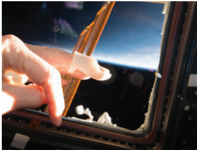
FIGURE 2. A finger splint designed by Dr. Julielynn Wong was manufactured by the Additive Manufacturing Facility (AMF) onboard the International Space Station. (Image credit: NASA)
