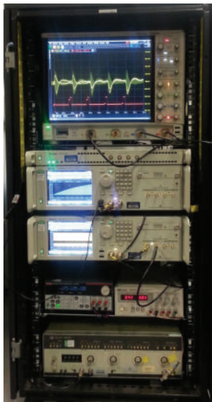
FIGURE 3. Current QKD systems use bulky rack-mounted equipment as shown, but smaller and even chip-based systems are envisioned and in development. (Image credit: Rupesh Kumar/University of York)
