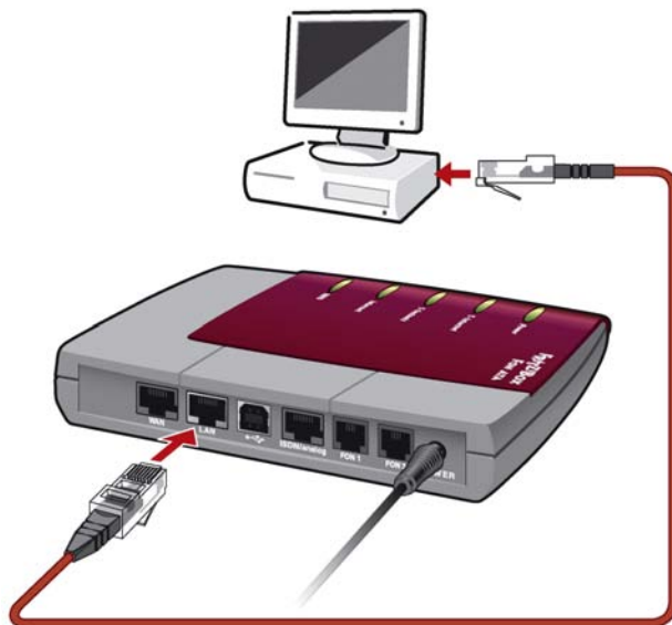
Connecting FRITZ!Box Fon ata to a computer's network adapter
