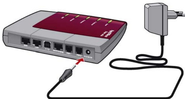
Connecting FRITZ!Box Fon ata to the power supply
